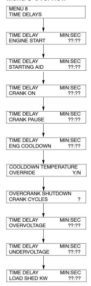
If the Cooldown Temperature Override is not enabled, the unit will cease to run when the engine temperature falls below the ENGINE COOLED DOWN temperature (shown in Menu 2).
